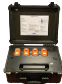
Bump/Cal Test Station
